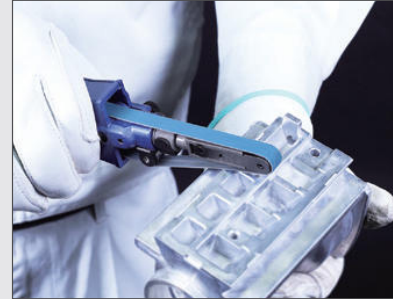
Chamfering of straight parts.
