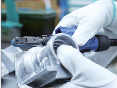
Deburring of die cast parts.
