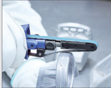
Detail finishing of aluminum material.
